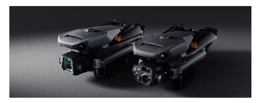
The Mavic 3 Enterprise redefines industry standards for small commercial drones. With a mechanical shutter, a  $56 \times$  zoom camera, and an RTK module for centimeter-level precision, the Mavic 3E brings mission efficiency to new heights. A thermal version is available for firefighting, search and rescue, inspection, and night operations.
